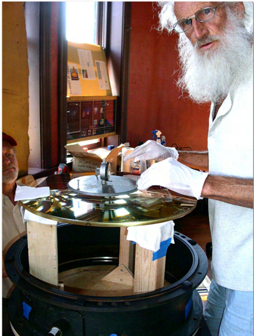
Jack carefully (very carefully) sets the spherometer on the lens surface to measure the radius of curvature of the Crown lens element.
